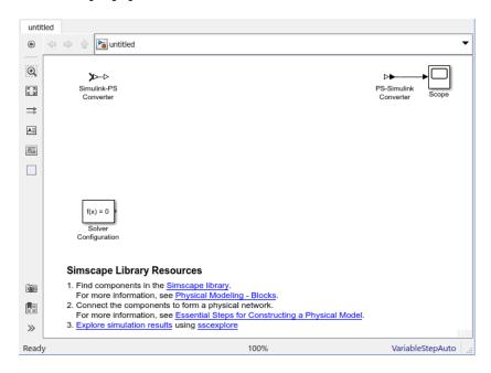
By default, the model name is not specified, the model contains a Solver Configuration block, a Simulink-PS Converter block, and a PS-Simulink Converter block connected to a Scope block. The default solver is VariableStepAuto. The resources section at the bottom of the model window provides links to the relevant block libraries and documentation topics.
